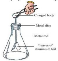
It consists of a metal rod. At one end of the rod, two leaves of aluminium foil are fixed and at the other end, there is a metal disc. The leaves of aluminium foil are placed inside a conical flask and the flask is corked to isolate the leaves from air.
